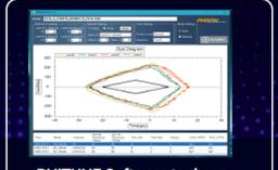
PHITUNE Software tool can automatically set different gain parameters in the Redriver for the customer's development environment.
