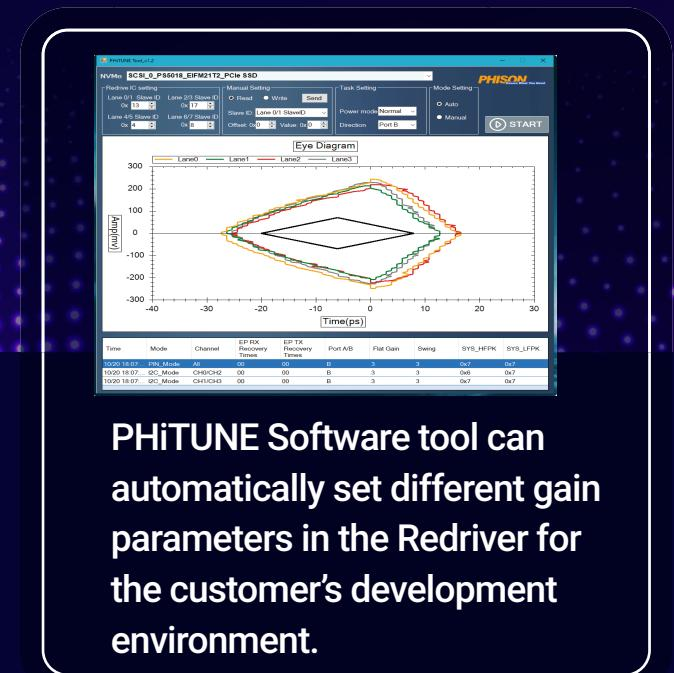
PHiTUNE Software tool can automatically set different gain parameters in the Redriver for the customer's development environment.
