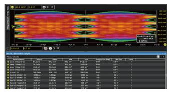
PS7162 measurement result in a PCIe 6.0 (PAM4) system environment.
