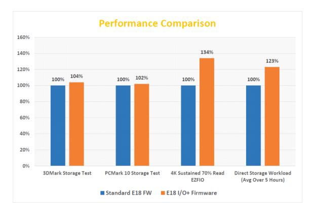
The standardized tests in the chart above show examples of what to expect with a 2TB PS5018-E18 SSDs. End users will see a small performance increase in existing consumer-level workloads. Next-generation workloads that stream data see the largest performance increase.
