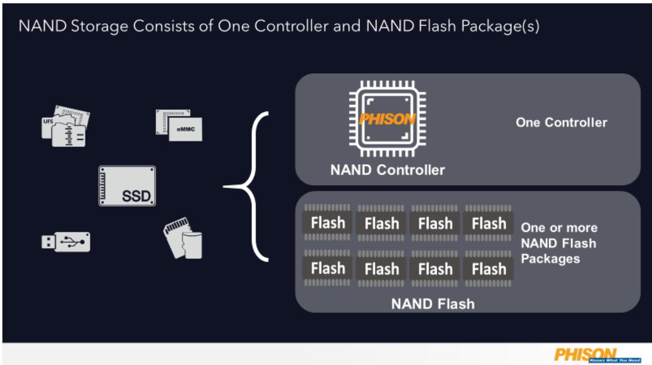
Exhibit 1: Typical internal construction of a NAND storage device
